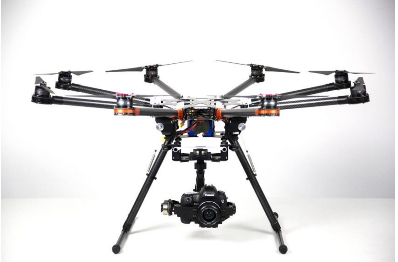
DJI S-1000 with large camera and gimbal
