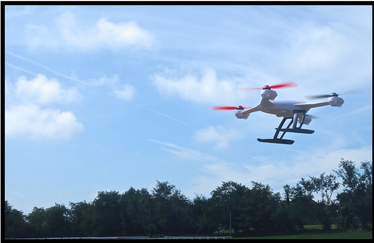
Blade 350QX Quadcopter - note the 4 propellers
